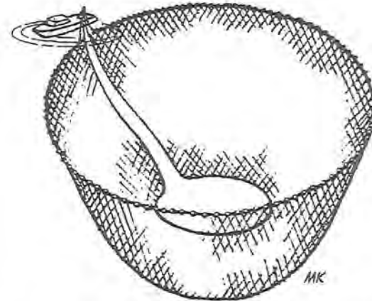
Figure 12.6: A purse seine net set from a tuna fishing vessel (top left-hand corner).
